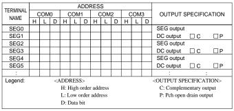
Multiple specifications are available in segment option item as indicated in the following example. Using "S5UC62xxxD Manual" as reference, select the specifications that meet the target system and check the appropriate box. Be sure to record the specifications for unused ports too, according to the instructions provided.
